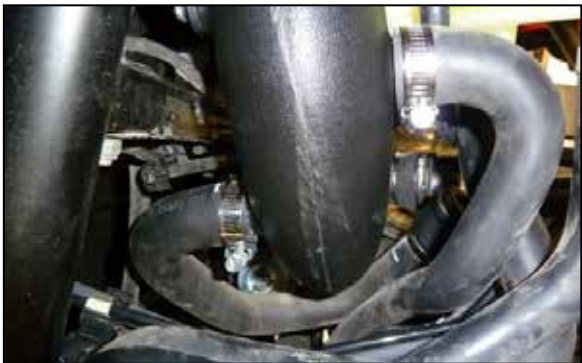
36. Install the vent lines onto the intake tube and secure with the provided hose clamps.
