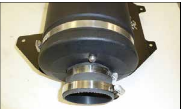
29. Install the provided coupler onto the filter housing inlet and secure with the provided hose clamp.
