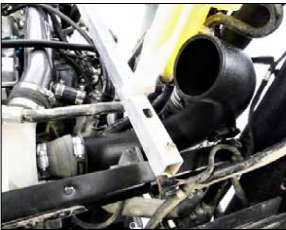
22. Install the K&N intake tube into the coupler at the turbo inlet but do not tighten the hose clamp at this time.
