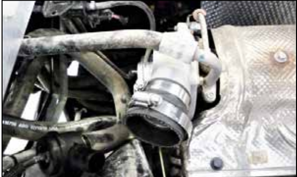
16. Install the provided step coupler onto the turbo outlet and secure with the provided hose clamp.
