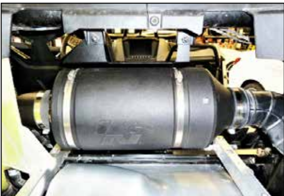
33. Install the fresh air intake duct onto the housing inlet and secure with the provided hose clamp. Note: for 2021 and later models, see steps 33a. through 33c.
