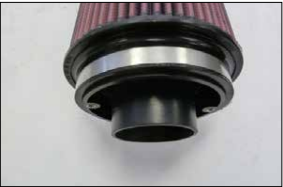
23. Install the radius filter adapter into the K&N air filter and secure with the provided hose clamp.
