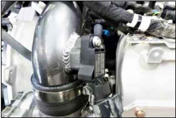
18. Install the Charge pipe sensor into the K&N charge pipe and secure with the provided hardware. Reconnect the electrical connection.
