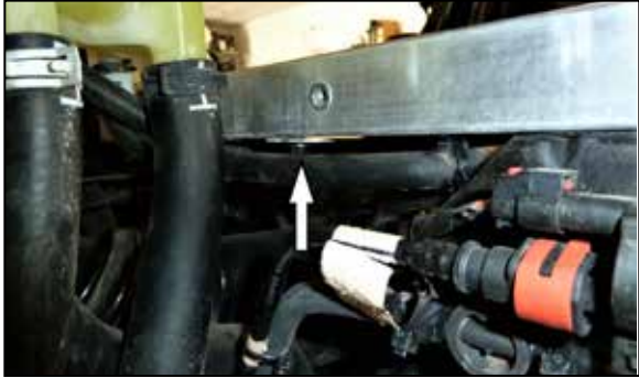
9. Remove the last remaining heatshield bolt shown and then remove the heat shield by sliding it to the right and then out.
