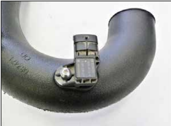
21. Remove the sensor from the factory intake tube and then install it into the K&N intake tube using the provided hardware.
