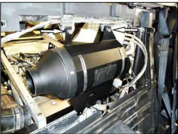
30. Install the filter housing assembly into position using just the upper mounting bolts, do not tighten the bolts.
