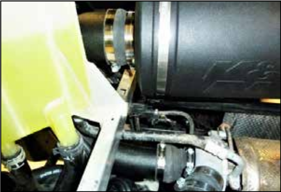
31. Install the intake tube into the coupler on the housing, align for best fit and then tighten both hose clamps.
