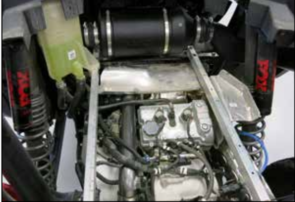
33c. Reinstall the fresh air intake duct and secure it the air filter housing using the provided hose clamp.
