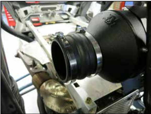
33b. Install the provided hump coupler onto the filter inlet and secure with the provided hose clamp.
