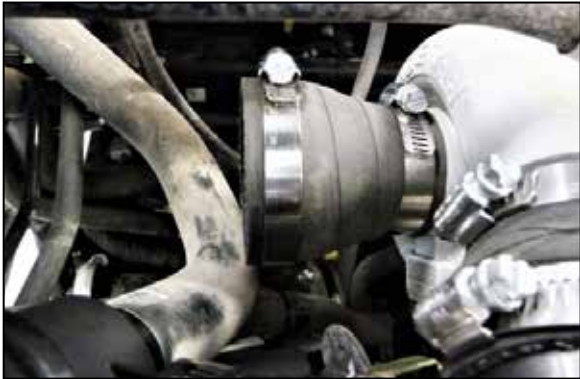
20. Install the provided step coupler onto the turbo inlet and secure with the provided hose clamp.
