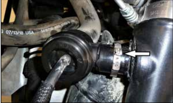
12. Loosen the one-time use clamp that secures the BOV to the charge pipe and then separate the BOV from the charge pipe.
