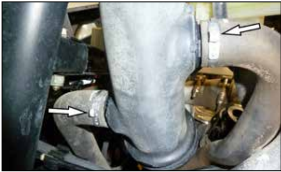
11. Loosen the two one-time use clamps that secure the vent hoses connected to the intake tube. Then disconnect the vent tubes from the intake tube and remove the intake tube from the vehicle.
