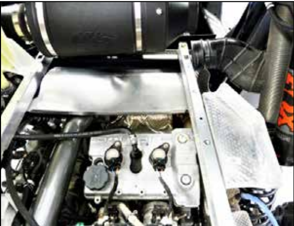
32. Reinstall the factory heat shield, secure the canister and heat shield with the provided and factory hardware. Note: Fully tighten all hardware.
