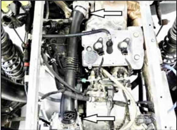
14. Loosen the hose clamps that secure the charge pipe and then remove the charge pipe from the vehicle.
