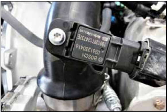
13. Remove the bolt that secures the charge pipe sensor and then remove the sensor from the vehicle.
