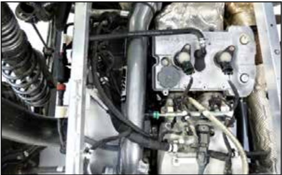
17. Install the K&N charge pipe, adjust the pipe for best fit and then secure with the provided hose clamp.
