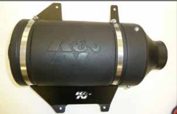
28. Install the filter housing onto the mounting bracket and secure with the provided hose clamp.
