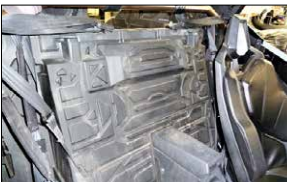
34. Reconnect the IAT sensor electrical connection and then reinstall the access panel and secure with the factory quarter turn fasteners.
