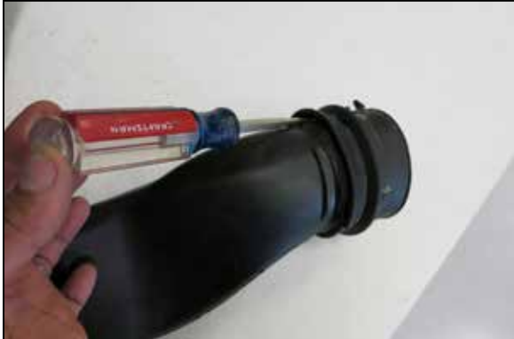
33a. On 2021 and later models it will be necessary to remove the complete fresh air supply duct from the vehicle and then remove the coupler adhered to the duct using a knife or screwdriver. It may also be helpful to use a heat gun.
