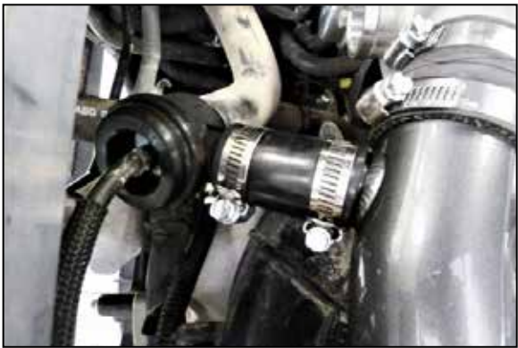
19. Using the provided hose and clamps, connect the BOV valve to the charge pipe.
