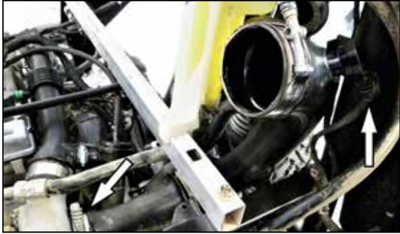
10. Loosen the hose clamp the secures the intake tube to the turbo and then disconnect the sensor electrical connection.
