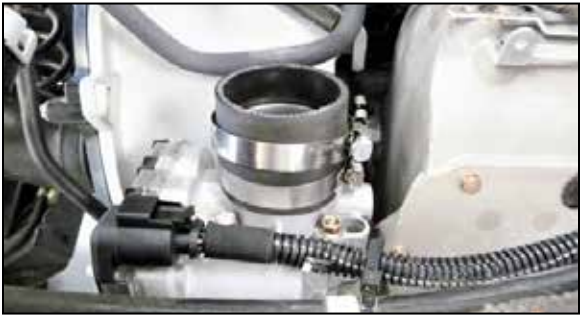
15. Install the provided coupler onto the throttle body and secure with the provided hose clamp.
